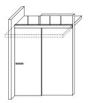
Width calculations W panel = W door space + 3 cm Height calculations H panel = H Floor/Under-rail (see page 67) - 1,8 cm
