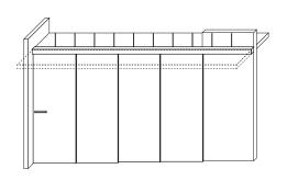
Width calculations W panel = W door space + 19,5 cm : 4 Height calculations H panel = H Floor/Under-rail (see page 67) - 1,8 cm
