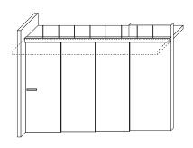
Width calculations W panel = W door space + 14 cm : 3 Height calculations H panel = H Floor/Under-rail (see page 67) - 1,8 cm
