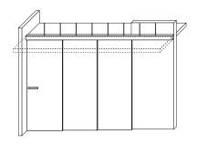
Width calculations W panel = W door space + 14 cm : 3 Height calculations H panel = H Floor/Under-rail (see page 67) - 1,8 cm
