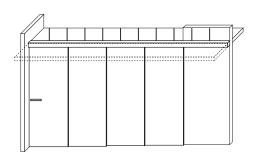
Width calculations W panel = W door space + 19,5 cm : 4 Height calculations H panel = H Floor/Under-rail (see page 67) - 1,8 cm
