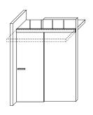
Width calculations W panel = W door space + 3 cm Height calculations H panel = H Floor/Under-rail (see page 67) - 1,8 cm
